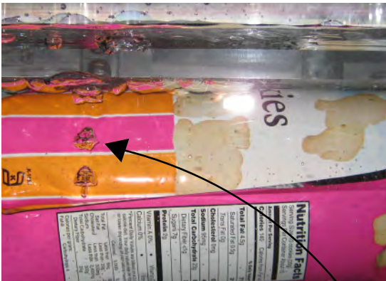
Faulty Seal - See The Air Bubbles!
