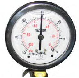
Adjust Vacuum Level to Evaluate Seal Integrity
