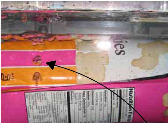
Faulty Seal - See The Air Bubbles!
