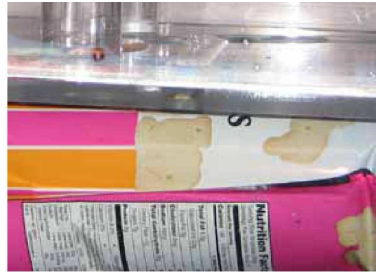
Good Seal Integrity - No Bubbles!
