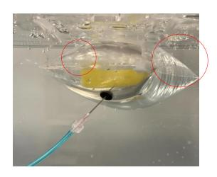
**Step 12:** Turn of the Vacuum generation, remove the package from the tank and carefully remove the needle. At this time proceed back to step 1 for the next package.
