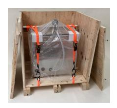
**Step 4:** If relocating the Leak Detector, use a pallet jack to lift the crate to move to the desired location, keeping the Leak Detector strapped to the crate while moving. Once in the desired setup location, remove the strapping securing the Leak Detector to the crate.
