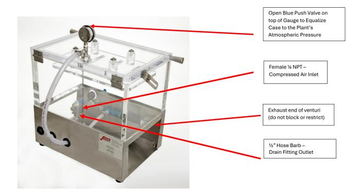
Air supply inlet on the Leak Detector is a ¼" NPT fitting (G-fitting adapters provided outside of North America)
