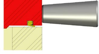
• Compress the seal into the groove. No adhesive is required. If seal is cut properly the compression of the butt joint will be adequate to seal properly.
