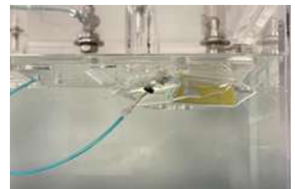
#6: Close lid so that package is submerged in water and held under the hold-down plate.
