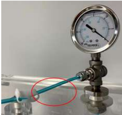
#1: Ensure that the white clamp attached to tubing (top of tank's lid) is closed (depressing tube).
