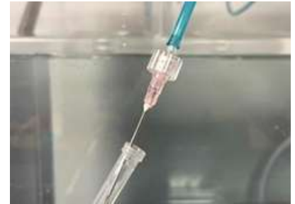
#3: Remove cover from needle. PLEASE NOTE: While the cover is over the needle, turning clockwise will tighten the needle in the tubing adapter fitting. Twisting the cover counterclockwise will loosen the needle. Ensure the needle is secure in the fitting.
