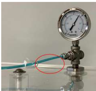
#8: Adjust Vacuum Level till Vacuum Gauge (on top of the Lid) reaches the desired test level.
