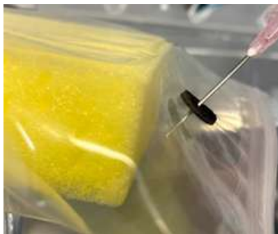
#4: Carefully insert needle into septum. Ensure the needle does not puncture the opposite side of the package or into product.
