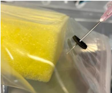
**#4:** Carefully insert needle into septum. Ensure the needle does not puncture the opposite side of the package or into product.
