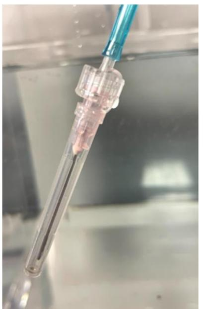
**#13:** When testing is complete, ensure the needle cover is reinstalled on the needle.
