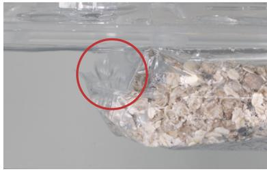
**Step 5: Monitor Sample for Leaks**
