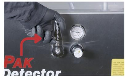
**Step 6: Turn off Vacuum System & Complete Test**
