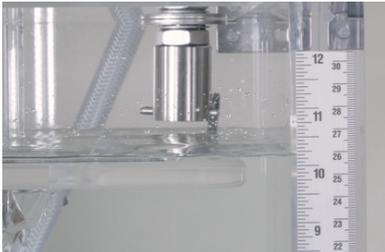
**Step 1: Fill Leak Detector with Water**
